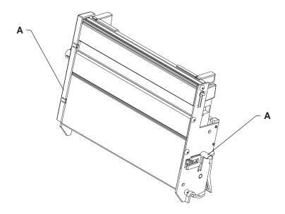
When you reinstall the ASF, be sure the feed arm assembly is vertical, with the feed pawl at the top.
